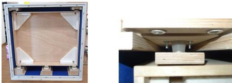
**Fig. 10** Box-in-box transport case [38] **Fig. 11** Support between inner and outer case [38]
